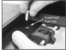
D. Hold bolt at top and tighten nut under side rail. Repeat Step 5C and 5D for right tension adjuster.
