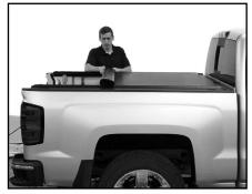
D. On both sides, seal cover edges with hook and loop system the full length of cover.
