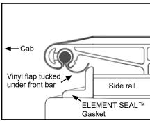
F. With the tension adjuster's support tab under the side rail, tighten bolt (left loose earlier) under front bar on each tension adjuster.
