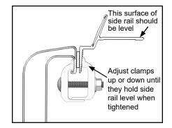
E. Install second clamp on side rail at midway point. Adjust side rail until flush at top and then repeat clamping procedure.
