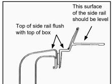
C. Install first clamp as close to front of box as possible and then use 1/2" wrench to tighten.
