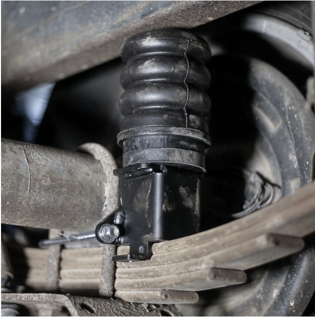
TRAILER SUMOSPRING INSTALLED
