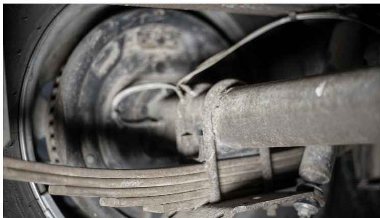
FACTORY GAP BEFORE TRAILER SUMOSPRING INSTALLATION
