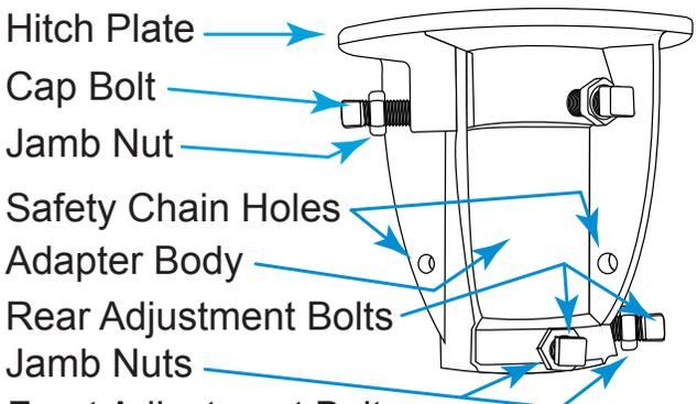
To prepare, move the Jamb Nuts out to the head of the Cap Bolts. The adapter body weighs over 50 lbs, so an additional person may be required to help. Slide the Adapter Body up over the Locking Collar, with the "Front" label facing towards the cab of the vehicle. Begin tightening Cap Bolts evenly, making sure the adapter body is moving upwards, until firmly against the pin box. Tighten down the Cap Bolts to approx. **110 ft. lbs.** Tighten jamb nuts firmly.
