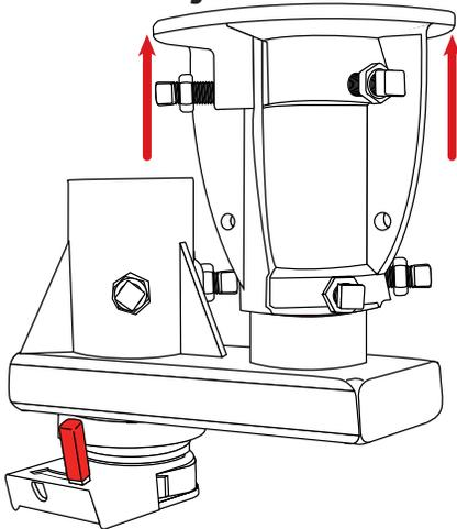
To set the C5GX1216 from 12 to 14 inches, loosen the rear adjustment bolts and lift the Adapter Body up.
