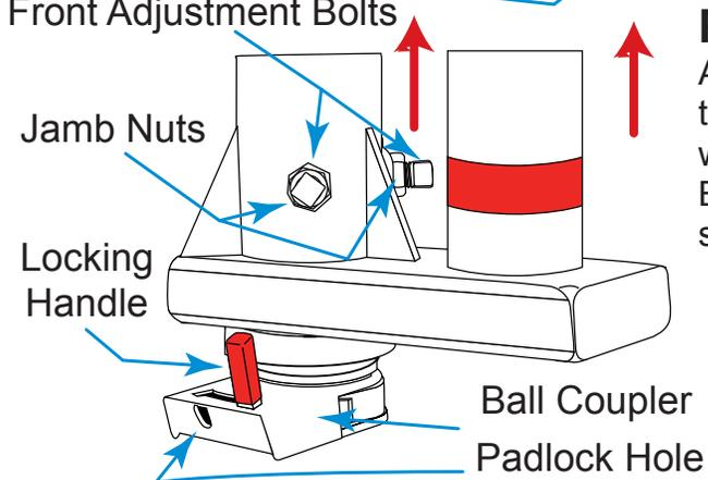
Align the Ball Coupler Platform so the FRONT Label facing towards the cab of the vehicle. Slide the Ball Coupler's pipe with the red stripe into the Adapter Body until it touches the Ball Coupler Platform. Tighten the Rear Adjustment Bolts, securing the Adapter Body to the Ball Coupler Platform.
