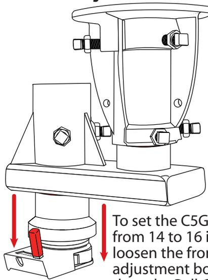
To set the C5GX1216 from 14 to 16 inches, loosen the front adjustment bolts and drop the Ball Coupler down.
