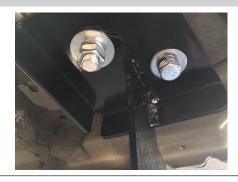
Starting on the driver-side front mounting point, use a flathead screwdriver to remove the hole plug on the outside of the vehicle and insert an M8 bolt plate and plastic bolt retainer to hold the bolt in place.
