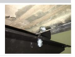
To finish installing the front mounting bracket, remove the factory hex bolt towards the center of the vehicle.
