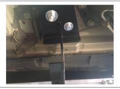
Before placing the running board onto the mounting brackets, place a running board spacer bracket onto each of the mounting brackets.
